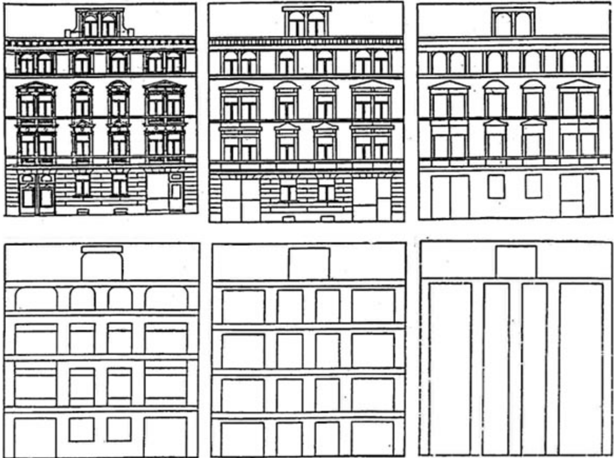
Fig 1. Stages in information reduction of a typical German townhouse facade. After BUTTLAR, 1973.
